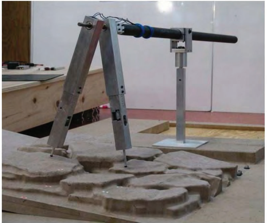
Figure 7-3: Compass gait robot posed on rough terrain.
